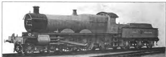
Fig. 5053. Ten-Wheel, Four-Coupled Locomotive. Great Western Railway. Cylinders 18 in. x 30 in.; Working Steam Pressure 225 lbs. per sq. in.; Total Heating Surface 2,142.9 sq. ft.; Weight on Drivers 79,750 lbs.; Total Weight 106,400 lbs.
